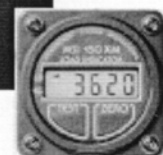
Cargo hook scales consist of a load-sensing device and an instrument-panel meter.
